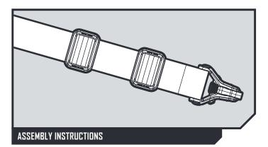
To connect the *Paraclip* to the sling, run the end of the *MS1* through the *Paraclip* and then back through the *Fit Buckle*(s). Double the *webbing* back through the upper *Fit Buckle* if possible.
